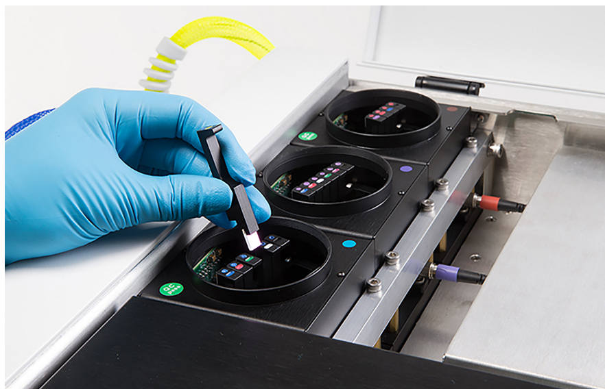
Figure 3. The three detection modules of a 3-laser, 13-color Beckman Coulter CytoFLEX flow cytometer. Each fiber-coupled module contains several compact dichroic filters on removable holders (like the one held up in the image) for spectral separation of signals.
